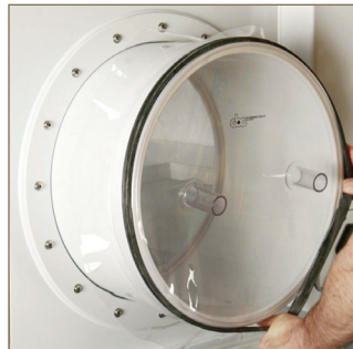
The photo sequence above shows a 18" diameter transfer port cap (flanged) with nipples being installed on a semi-rigid, germ-free isolator transfer port using a CBC Patent Clamp.*
