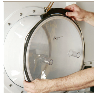
The photo sequence above shows a 18" diameter transfer port cap (flanged) with nipples being installed on a semi-rigid, germ-free isolator transfer port using a CBC Patent Clamp.*
