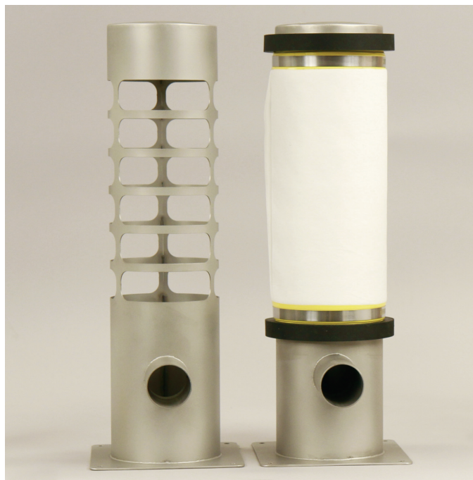
Pictured above are standard 5" (diameter) inlet filters used in our Isolators to help maintain a controlled, more uniform environment. (Filter on the left shown without filter media.)
