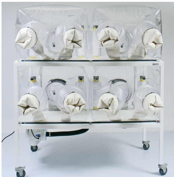
Pictured above is a positive pressure, germ-free, flexible film quad isolator showing pairs of independent glove extensions and 15 mil Hypalon/CSM dry box gloves
