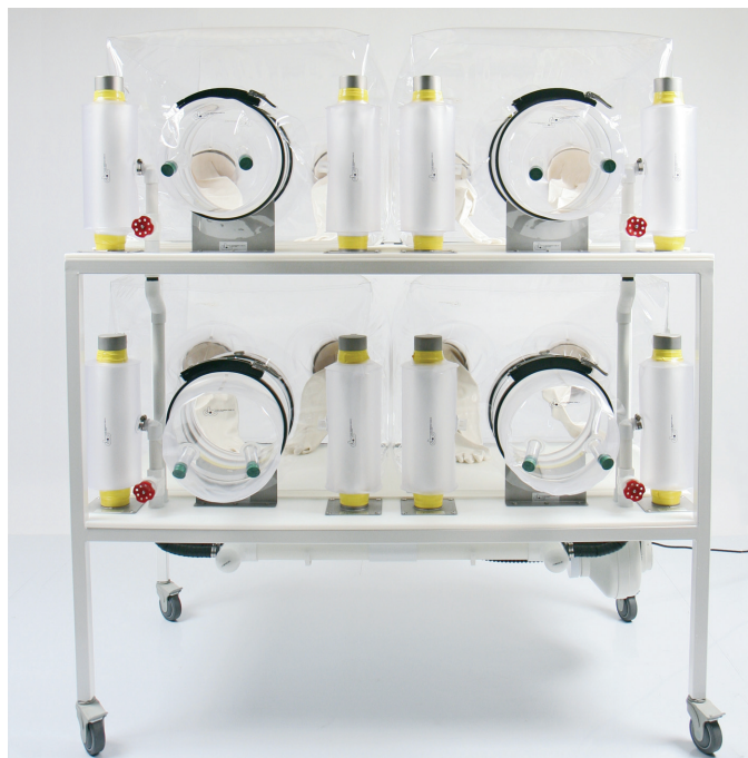
Pictured above is a positive pressure, germ-free, flexible film quad isolator showing independent transfer ports and 3" filter systems.
